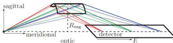
**Figure 1:** Schematic overview of the Von Hamos geometry for a XAS/XES spectrometer. Figure adapted from Anklamm et al.<sup>[1b]</sup>
