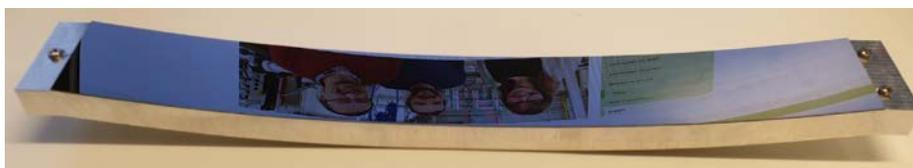
**Figure 1:** A ground-bent silicon crystal mounted on an aluminum support. The surface radius is 750 mm while the atomic planes are curved with a double radius. The crystal thickness is 300  $\mu\text{m}$ , the working surface is 300 mm  $\times$  38 mm.
