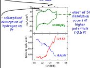
The change in diffracted intensity at reciprocal lattice positions of interest is monitored as the applied potential is cycled. The mirror like increase of intensity above the Bragg peak with decreasing intensity below is consistent with a changing expansion of the surface atomic layer.
