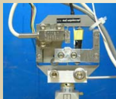
piezo stretching cell for in situ X-ray scattering on single fibres
