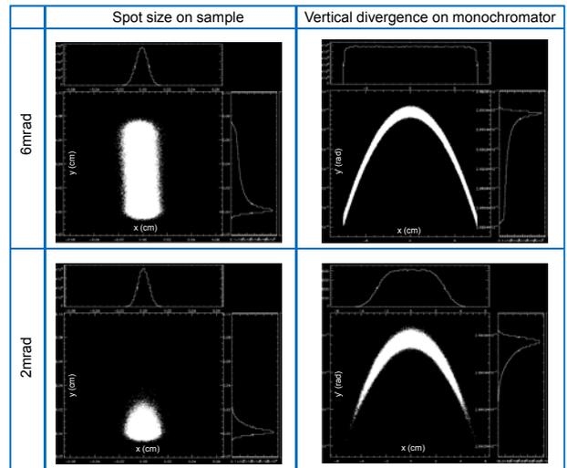
Vertical beam size contributes to spectrometer energy resolution.
