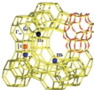
Fig. 2: Representation of the Y zeolite framework and cation location. In the fraction of the framework located in the upper right part of the figure O atoms are represented in red and the T atoms (Si or Al) in yellow. For clarity, in the remaining part of the framework, only yellow sticks have been adopted. Ag I cations are represented as spheres and are labelled with I, I', IIa, IIb and I' m . The supercage cavity, where guest molecules can be hosted, can be seen in the centre of the figure.
