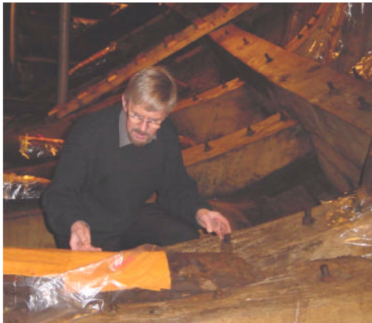
Magnus Sandström examining the poultrices for neutralisation of acid in the Vasa 's hold
