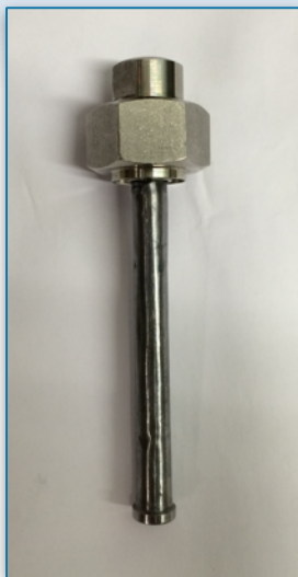
sample in a vanadium container V scatters only incoherently
