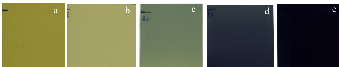
Figure 5. Examples of different blackening of the EBT3 films after one machine cycle. a) Film non-irradiated; b) Film with non-significant absorbed dose; c) Film from section 12; d) Film from section 11; e) Film from section 1.
