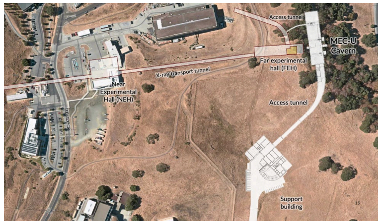
Figure 1: Location of the proposed MEC-U Cavern with respect to LCLS Near and Far Experimental Halls (NEH and FEH), as well as location of proposed MEC-U Support Building
