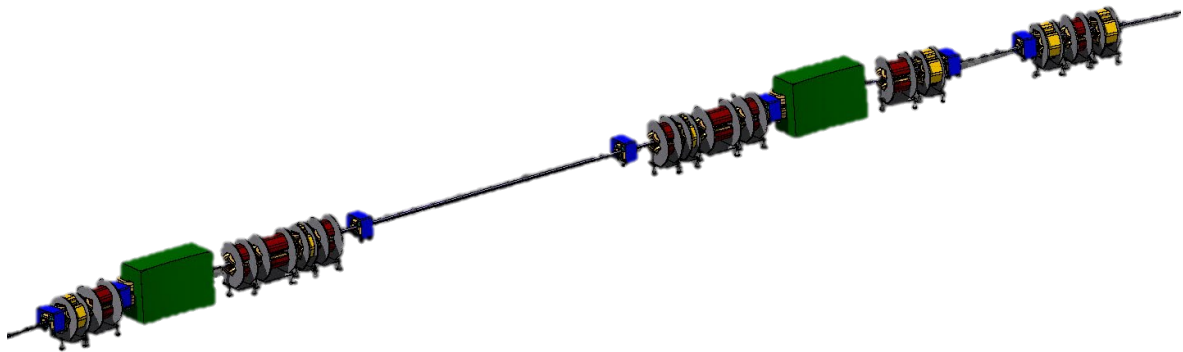
Figure 2. Fluka 3D model of a standard achromat, section 3.
