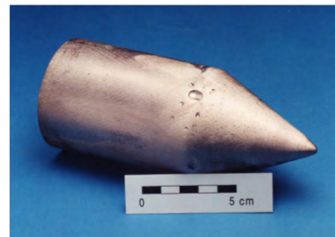
Heusler (Cu 2 MnAl) polarising crystal
