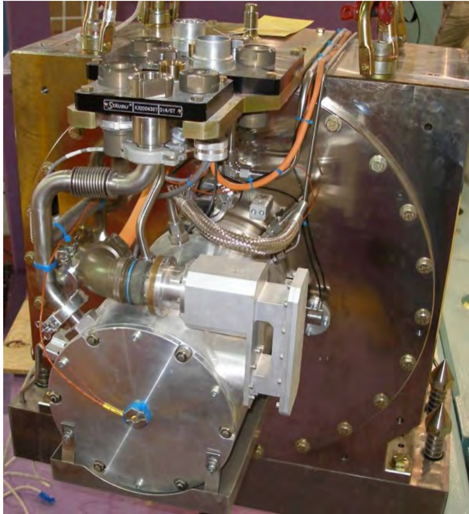
assembled T 0 chopper unit
