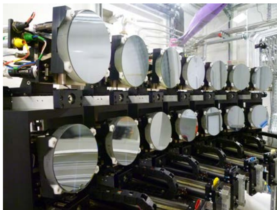
Figure 1: 14-crystal Crystal Analyzer Spectrometer on FAME-UHD beamline.
