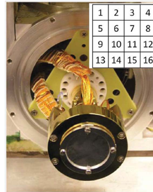
Fig. 2. The crystal holder mounted in the cryostat with an aluminum foil 10 \mu\text{m} thick acting as infrared radiation shield. The orange flat cables are the kapton insulated cables connecting the CPCB to the feedthroughs on the rear flange. The diagram shows the correspondence between channels and pads as the crystal is seen from the entrance window.
