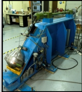
PYRENE 150 \text{ m/s} < V < 750 \text{ m/s} 35 \text{ g} < m < 60 \text{ g} bore \phi 32 \text{ mm}
