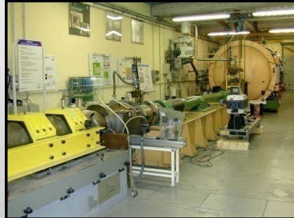
DEMETER 50 \text{ m/s} < V < 1000 \text{ m/s} 400 \text{ g} < m < 4000 \text{ g} bore \phi 110 \text{ mm}
