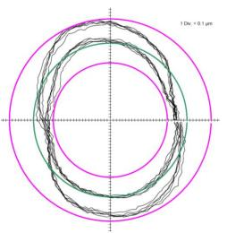
Air bearing with a SOC of 1.4μm
