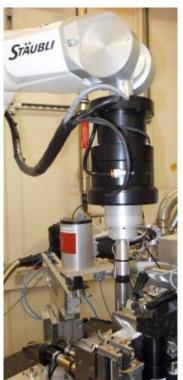
RoboDiff will be able to collect from any accessible orientation without deteriorating the SOC
