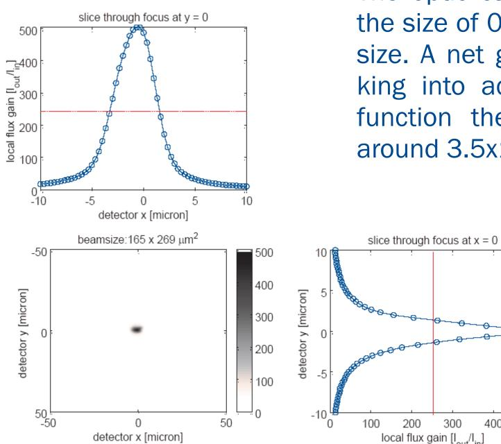
The optic can efficiently compress a beam of the size of 0.2x0.2mm<sup>2</sup> into a 4.5x2.5µm<sup>2</sup> spot size. A net gain of 500 was measured. By taking into account the detector point spread
