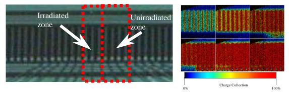
The proposed model of radiation damage of the n-Si strip detector for MRT dosimetry on ESRF synchrotron beam based on build up charge in a field oxide only has been proved. This model was successfully applied for explanation of the IBIC results. No bulk defect was observed that make detector radiation hard in this application. The build up charge effect can be avoided by overbiasing of the strips or by regular annealing under 150  $^{\circ}$ C if detector will be used in passive mode [2].
