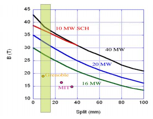
Preliminary field vs. coil gap and power for resistive and SCH magnets of various power levels.
