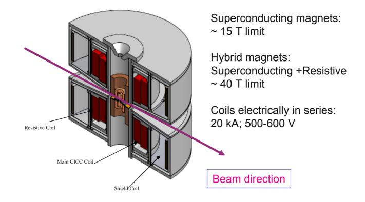
Section of the proposed split-coil, series-connected hybrid magnet
