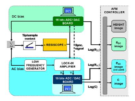
Figure 1 : Schematic view of the experimental set-up. The notations  $R_{DC}$  and  $R_{AC}$  indicate that resistance values can be obtained either from the "Resiscope" or from the lock-in, respectively. As improving the range and the resolution of  $R_{AC}$  is to the detriment of C measurement, we currently use a mix of DC for resistance and AC for capacitance imaging.
