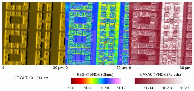
Figure 3 : Triple H-R-C maps obtained on the SRAM test sample supplied with Veeco's SCM system. sensors. This result proves that the capacitance image can be as rich and detailed as the resistance one.
