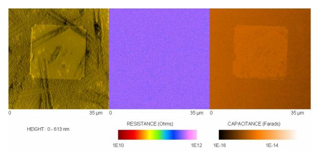
Figure 2 : Topography (left), resistance (center) and capacitance (right) pictures simultaneously recorded on a tiny square gold plate evaporated on a Macor® substrate ; the substrate backside is fully metallized to form a plane/plane capacitor. This is a typical example where the ohmic component is helpless to get any electrical information, whereas the capacitance image clearly reveals the pattern. Experimental parameters : tip/sample DC bias +1 V, AC bias 65 mV, frequency 10 kHz.
