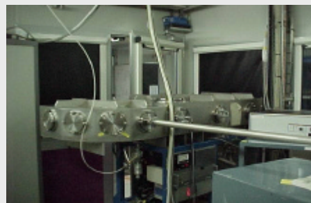
Fig. 1b: Photograph of the von Hamos spectrometer as installed at the ESRF beamline ID21.
