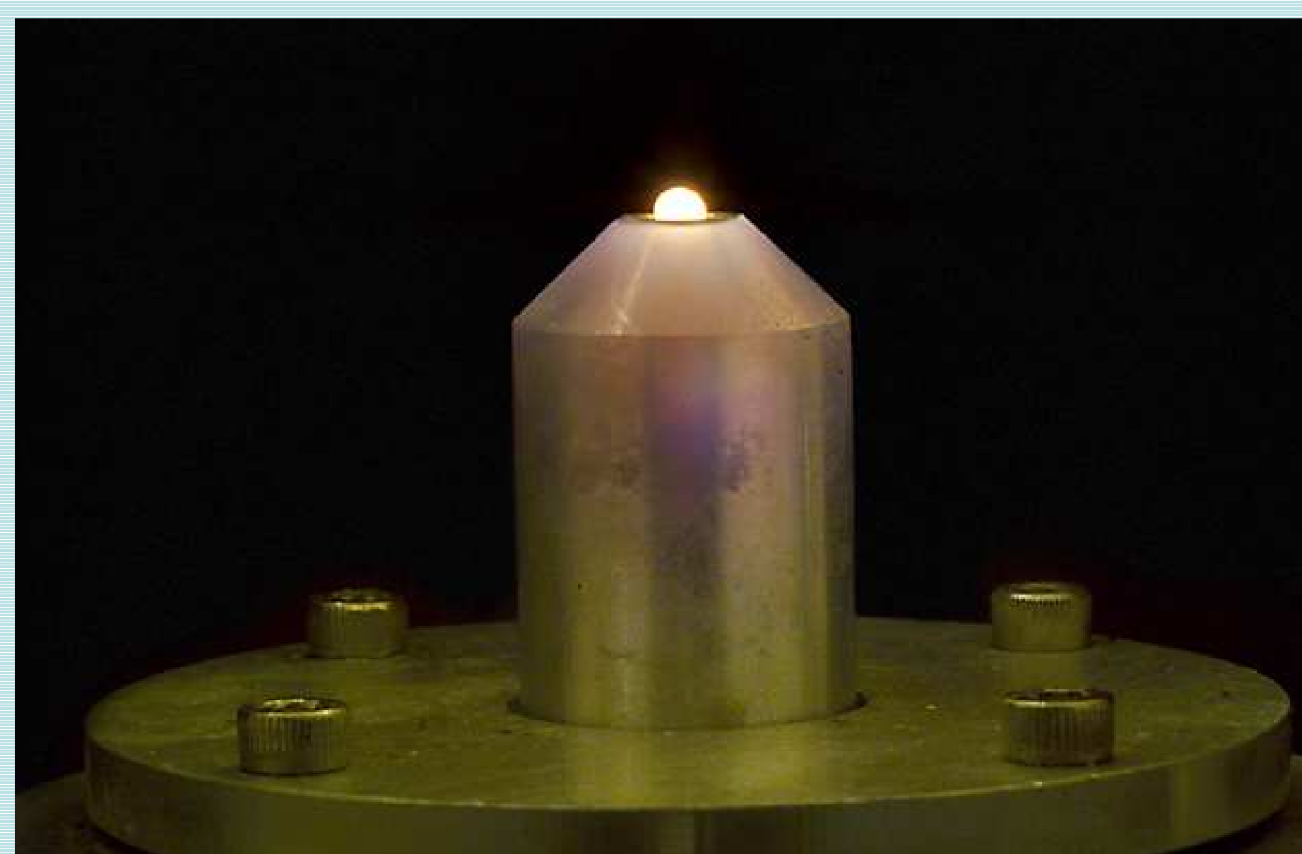
Figures 1-3: Left: Schematic view of levitation setup Middle: Levitated alumina sphere at 2100°C. The diameter of the sample is about 3 mm. Right: Integration of levitation setup at Sector 3, APS.
