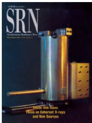
Figure 1a: Cryogenic STJ spectrometer with detector cold finger. Figure 1b: 9-Channel STJ fluorescence spectrum from a (biologically inactive) photosystem II protein (~100 ppm Mn). Figure 1c: Fluorescence-detected L-edge absorption spectrum from photosystem II
