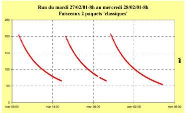
This system allows to enhance the beam lifetime and consequently instead of having 3 injections per day, we have only 2 injections a day.
