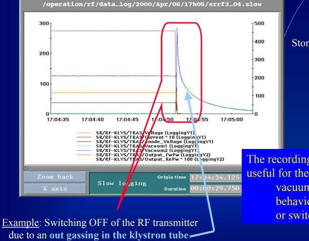
Storage of the evolution of all analog signals at 8Hz during 30 sec
