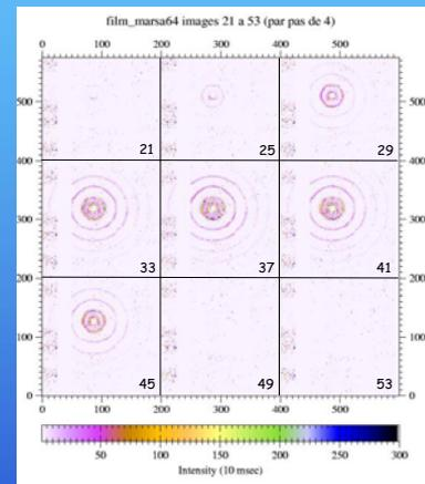
SAXS on Ag behenate (sample moving across the beam) exposure : 10 ms, time between images : 2ms, 64 images, 1 image/4 shown here (21 to 53)
