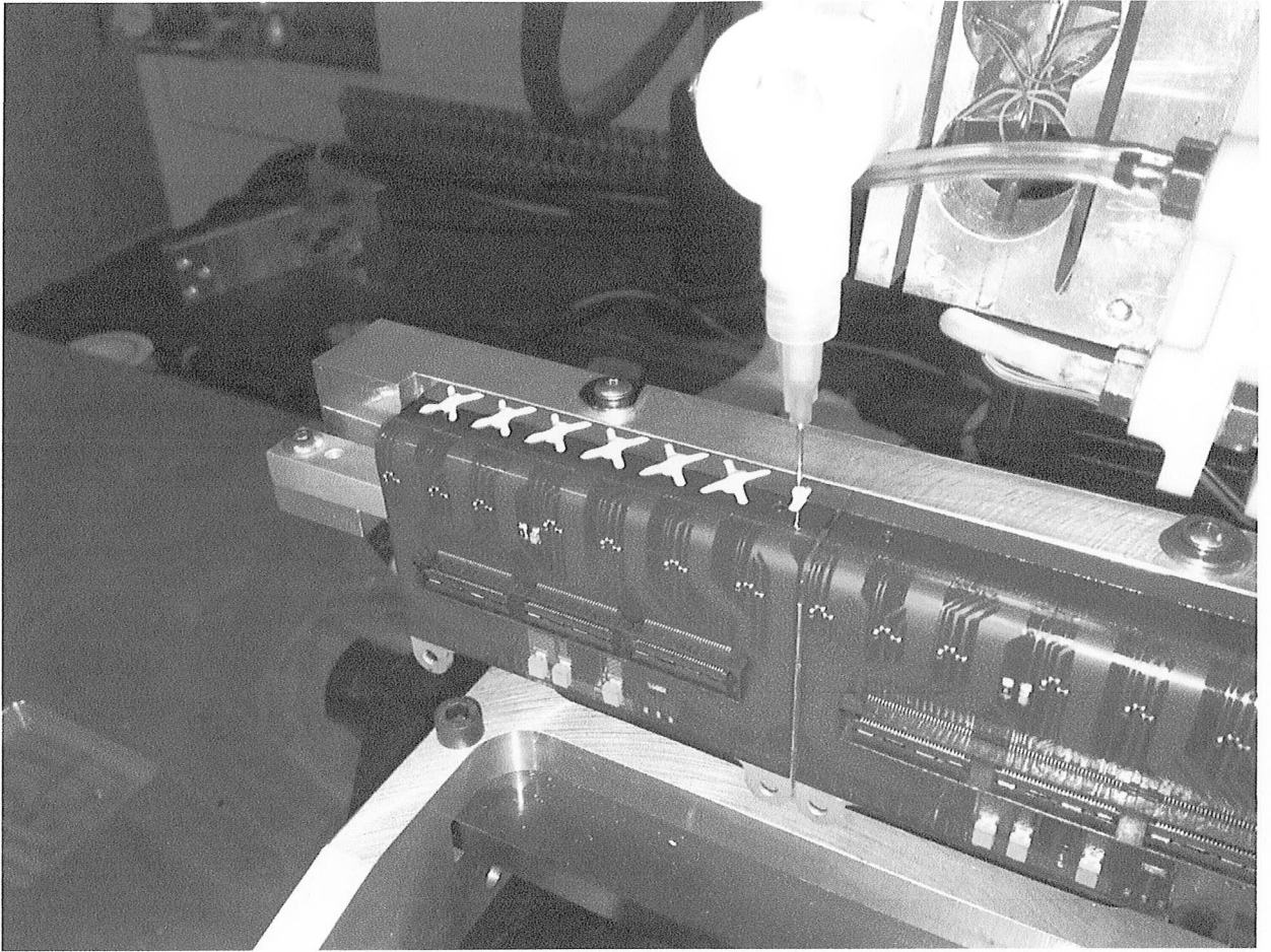
Figure 4.10. Glue deposition by the robot, controlling the volume as a function of the position.
