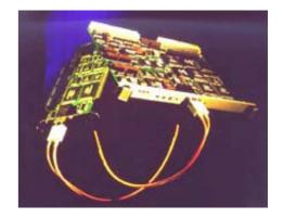
PCI – cPCI Bus Extender (MXI-3) NI PXI-PCI8330, Cooper link Transfer rate: 84 Mbytes/s
