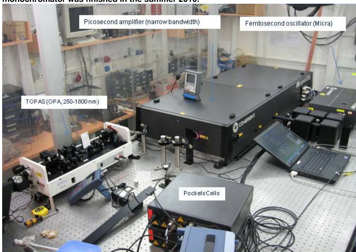
Figure 4a. Experimental table in hutch EH2 for pump-probe experiments. The multilayer monochromator was finished in the summer 2010.
